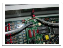
Correct connection of the OP232 to an S200-EC is shown to the left.
